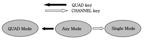
The following diagram shows the sequence of selected mode when pressing MODE key.
